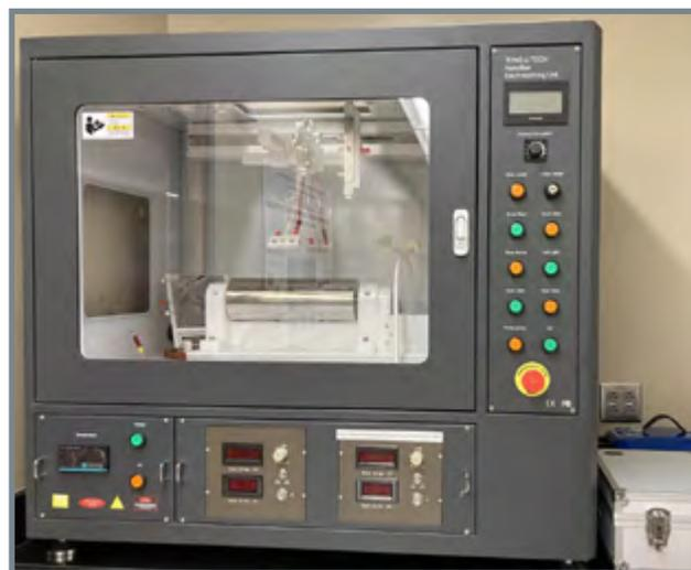
The electrospinner unit used to produce nanofibers.
